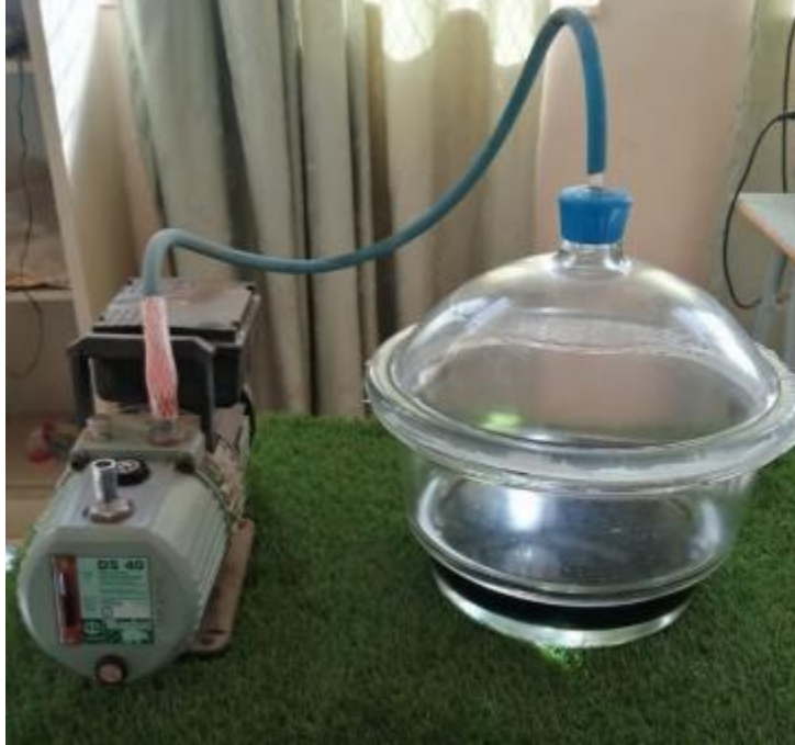
Figure 3. 29 Core samples oil saturation process
