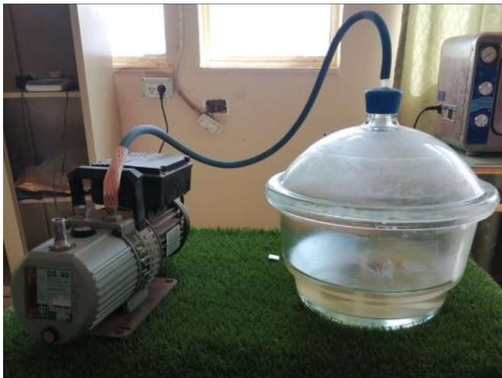
Figure 3. 27 Core samples reservoir water saturation process
