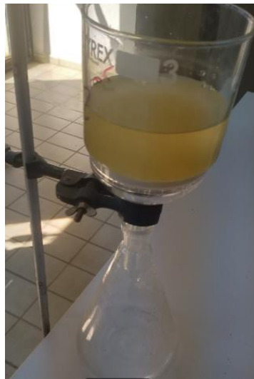
Figure 3. 17 Associated formation water filtration
