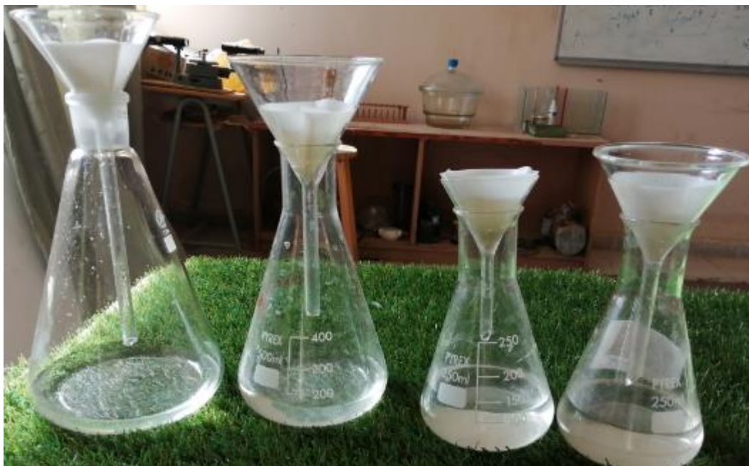
Figure 3. 23 Filtrating water from silica and zeolite
