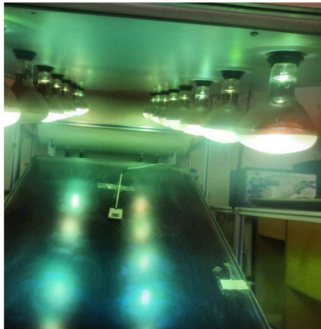
Figure 5.4 Absorber, sensors Using solarimeter, To measure the intensity of radiation
