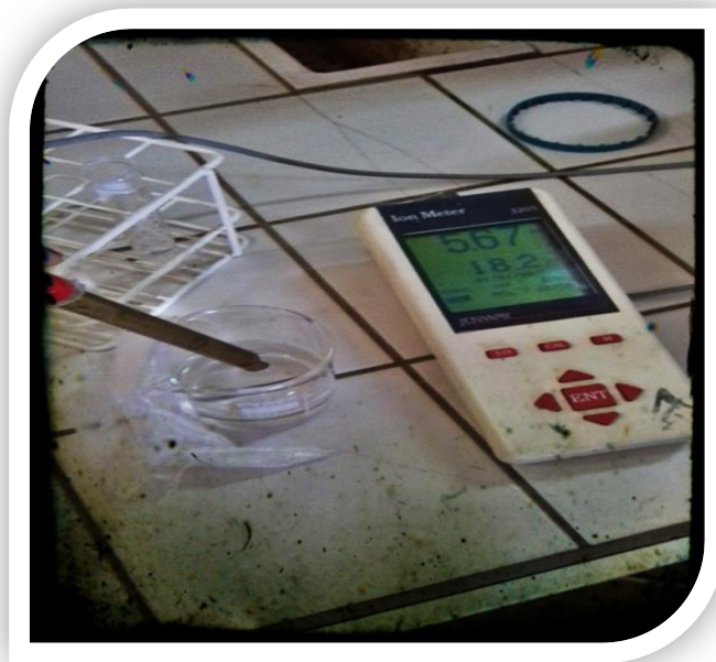
Figure 4.2. Put Small Sample in Baker 40ml.
