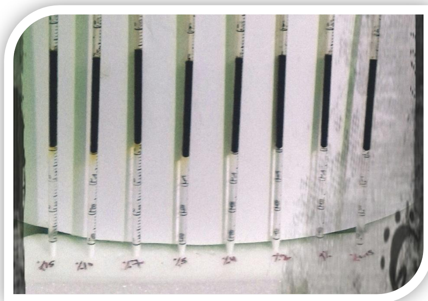
Figure 4.13. Injection the Surfactant and Oil.
