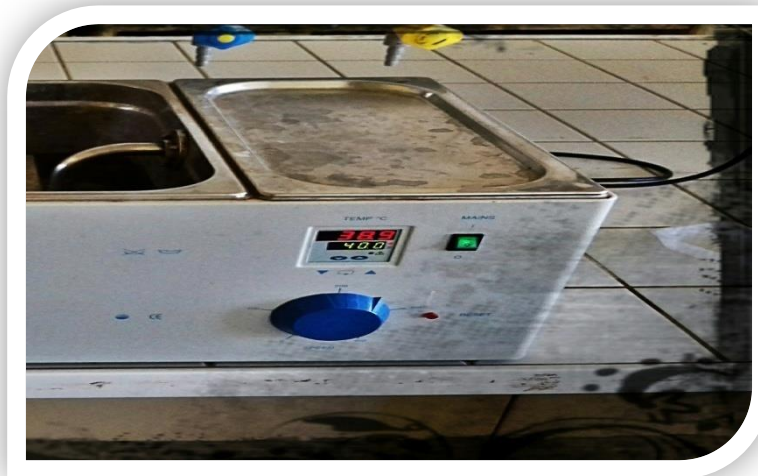
Figure 4.17. Turn Temperature and Mixing Button.
