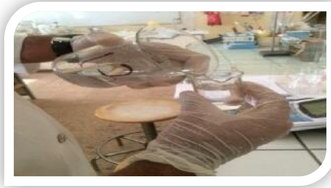
Figure 4.2. Put Small Sample in Baker 40ml.
