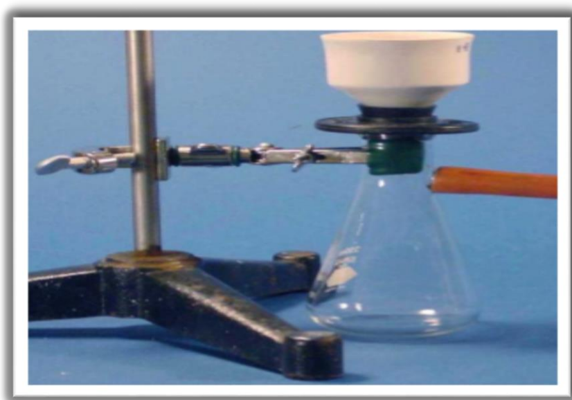
Fig 15 : Filtration By Buchner Funnel.
