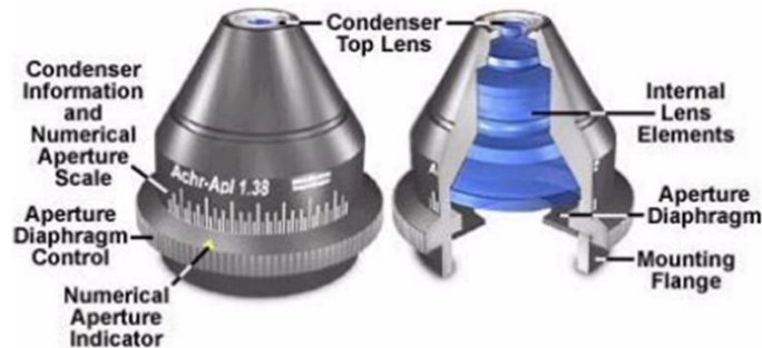
شكل (10) aplanatic-achromatic condenser
