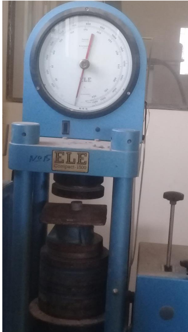
Figure 3.8. Compression Test Machine Used in the Present Work
